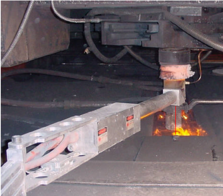
Figure 1: Laser Assembly – This model rides on a carriage that is extended over the mold while casting. The unit may be swiveled into practically any spot in the mold
