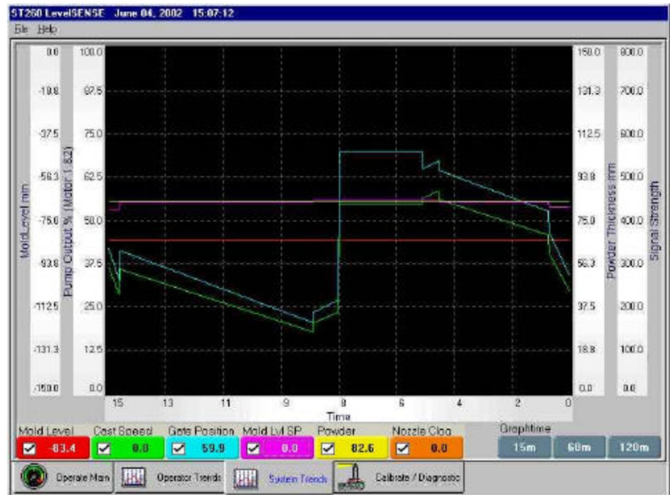
Figure 2: System Trending screen – monitor up to six system variables simultaneously, such as mold level, powder thickness, cast speed, gate position, surface temperature and others.
