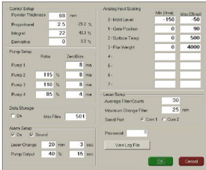
Figure 3: System Setup screen – important system control and process variables are easily modified to maximize operations.
