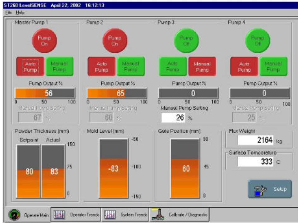
Figure 1: Main Operating screen – used for controlling the pumps, adjusting biased flow ratios, powder thickness Set point and alarm features.
