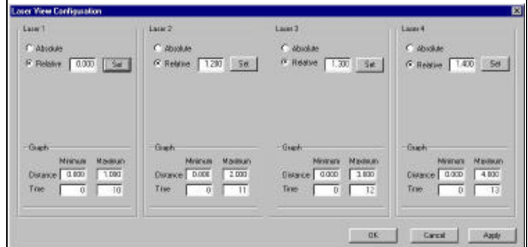
Figure 2: The configuration screen allows the user to set recording in either a relative or absolute mode with respect to the objects position as well as vertical and horizontal limits on the graphs.
