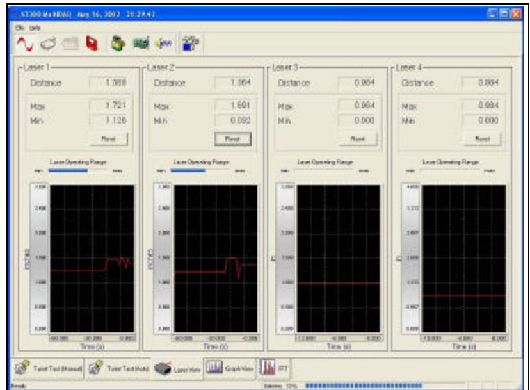
Figure 1: The LaserVIEW program is a versatile data acquisition tool that is used to capture displacement laser data and display the information on a laptop or PC. It is used in conjunction with the ST300 MTS portable data acquisition system.
